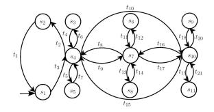
Figure 5: Finite State Machine for Channel Navigation
